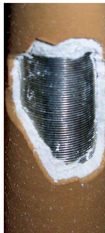
A sample of the uniformly floated individual layers of kieselguhr on the candle.
