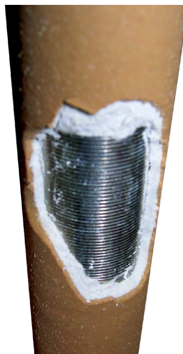
A sample of the uniformly precoated individual layers of kieselguhr on the candle.
