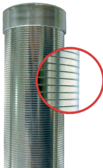
A detail of the candle slots between the turns of the trapezoidal wire (slot width 50 micrometers)
