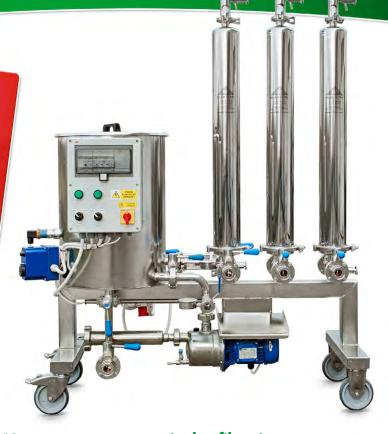
You can process particular filtration stages in one step and directly bottle
